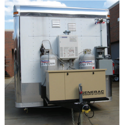
CPCC Welding Technology students designed and installed brackets to hold the generator and propane tanks
